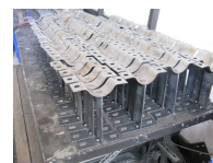
BRACKET SUSPENSION, TYPE B
